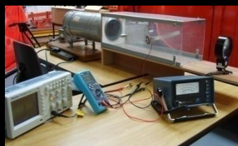
Fig. 3 Wind experiment setup Wind speed was measured using an anemometer placed 20 cm in front of the tunnel. Turbulence was created by a valve opening and closing mechanism.
