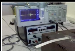
Fig 1. Rain drop experiment setup. Impact was induced by releasing water droplets from various heights.
