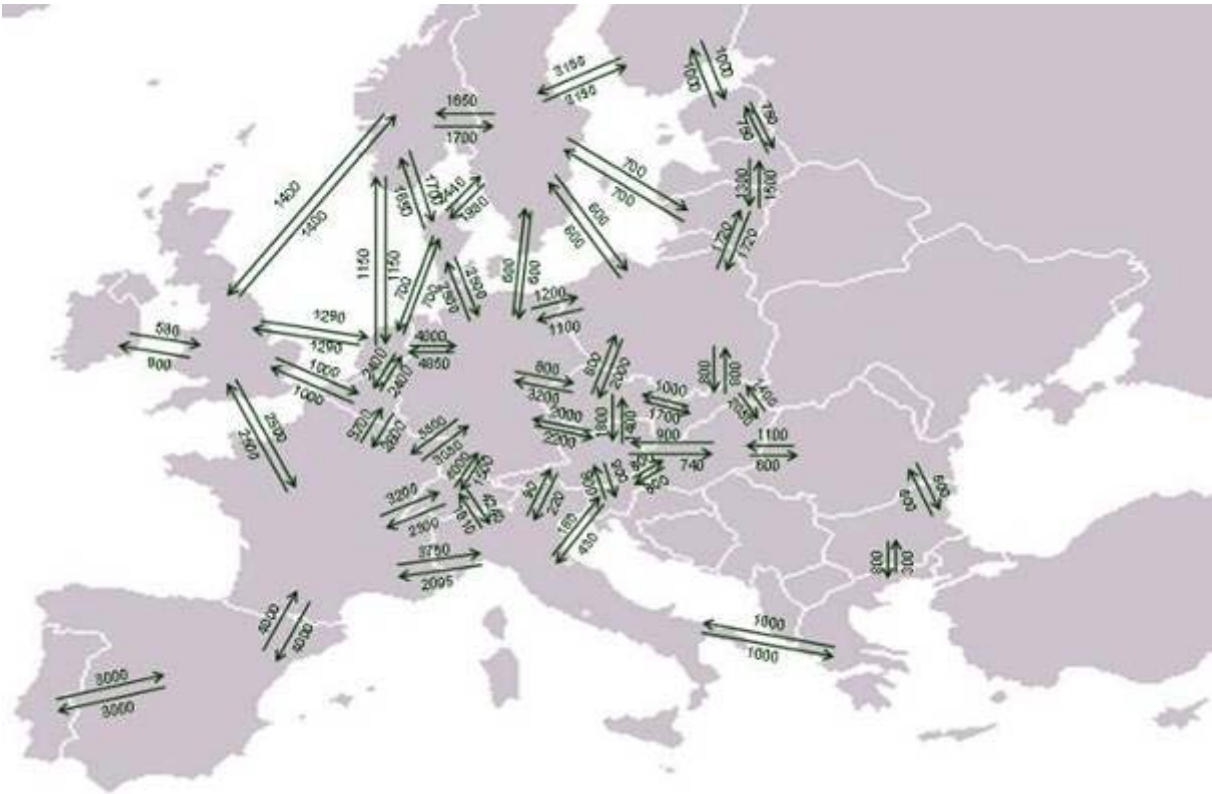
Map 6: Interconnection capacity requirements 2020 in MW 47 , PRIMES Reference scenario (source: KEMA, Imperial College London)
