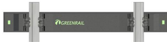
Figure 3: Greenrail sleeper (plan)
