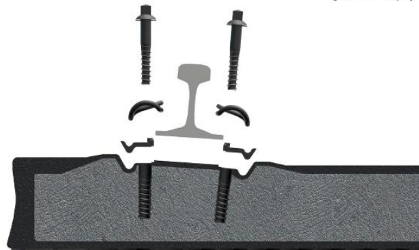
Figure 4: Greenrail sleeper (section)
